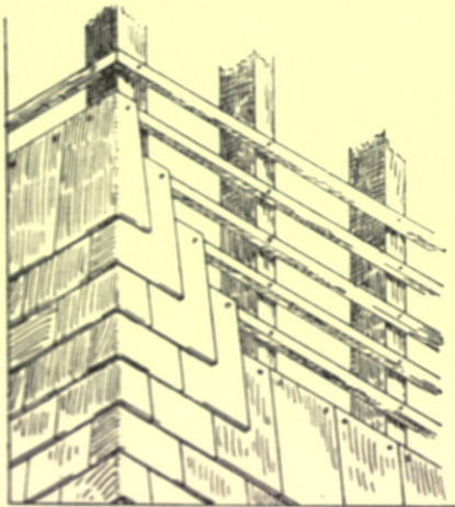
Fig. 54.—Timber-framed Wall covered with Weather-tiling.
